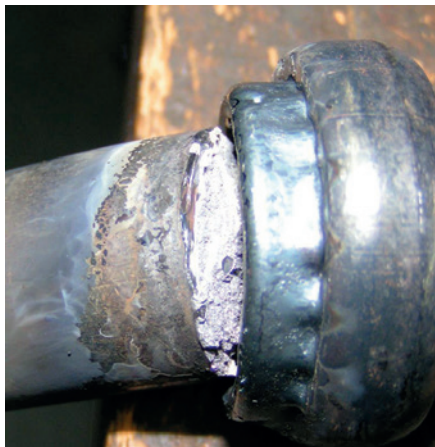
Fig. 3 • Small lack of fusion area at the edge due to a cold plunge, the stud does not reach the required 60° bending angle.
