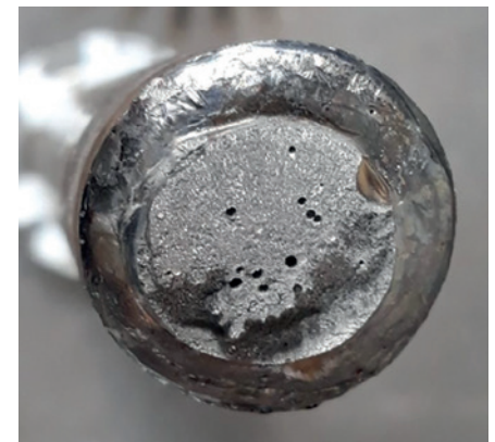
Fig. 5 • Massive lack of fusion at the edge due to a cold plunge, the weld zone breaks under low load.
