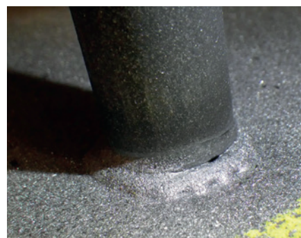
Fig. 4 • Undercutting caused by a plunge impediment.
