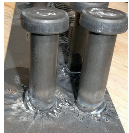
Fig. 15 • Welding results with the values shown in Fig. 14.
